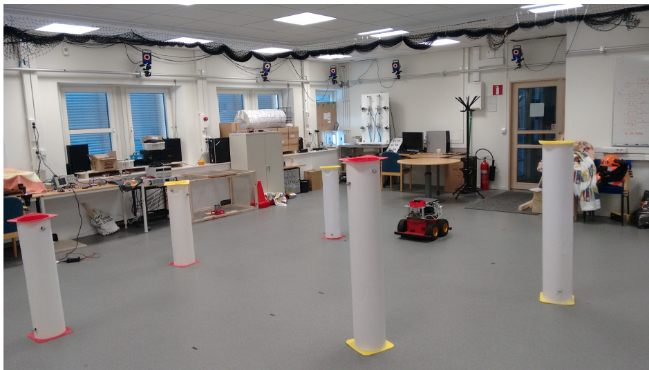
Figure 4. Setup of a typical calibration experiment, comprising five landmarks (white cylinders) and the robot-sensor system of Figure 3 moving among the landmarks.
